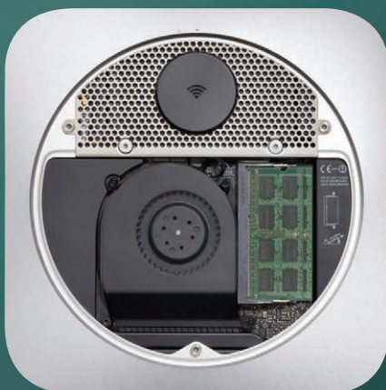
The new unibody mini provides a hatch on the bottom that you can quickly pop off to upgrade the RAM.
